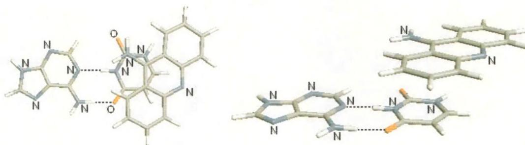
**Figure 3.5b**– The optimum stacked structure of 9-aminoacridine and AU base pair (AT-AD3) corresponding to MNDO method of calculation.
